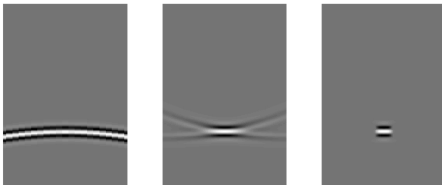
Figure: Simulations with noise free synthetic data: Left: Data. Middle: Reconstruction by Kirchhoff migration. Right: Reconstruction with sparsity regularization
