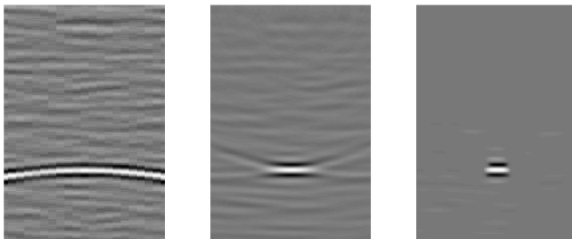
Figure: Noisy data. Left: Data. Middle: Reconstruction by Kirchhoff migration. Right: Reconstruction with sparsity regularization
